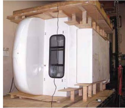
▲ Side load compression test set up
