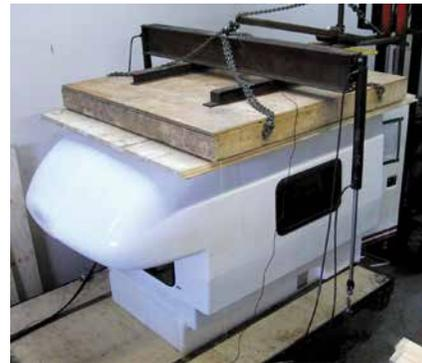
▲ Roof structural strength test set up
